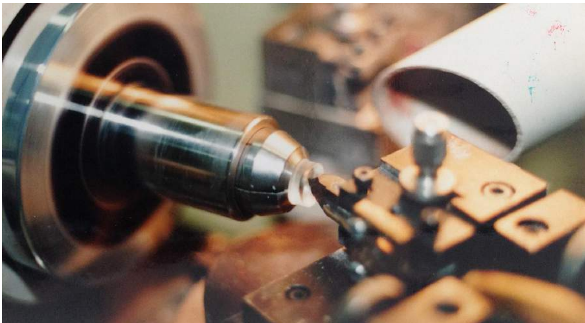
Diamond cutting tool shaping the surface of a contact lens button
