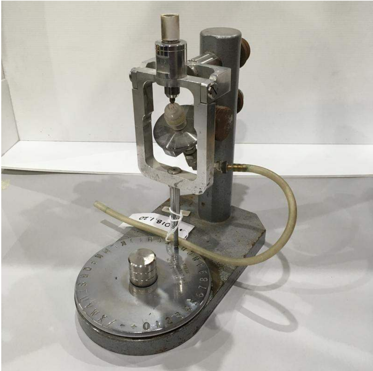
A pantograph which we used to engrave letters and numbers around the edge of a contact lens!
